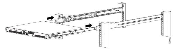
**3.** Slide the GSS and inner rails backward and forward in the two outer telescopic rail two or three times until the GSS seats properly in the rack.
